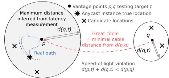
Figure 2: Analysis technique: anycast detection (figure adapted from [17])
